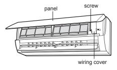
Make the power connection wire go through the cable-cross hole at the back of indoor unit and then pull it out from the front side.
