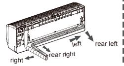
When select leading out the pipe from left or right, please cut off the corresponding hole on the bottom case.
